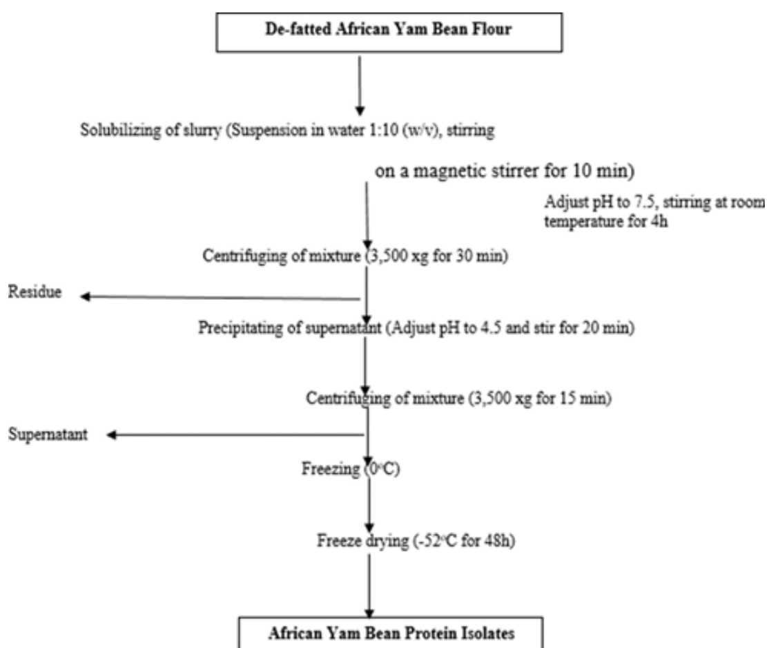
Figure 4. Flow chart for the processing of African Yam Bean Protein Isolates.
